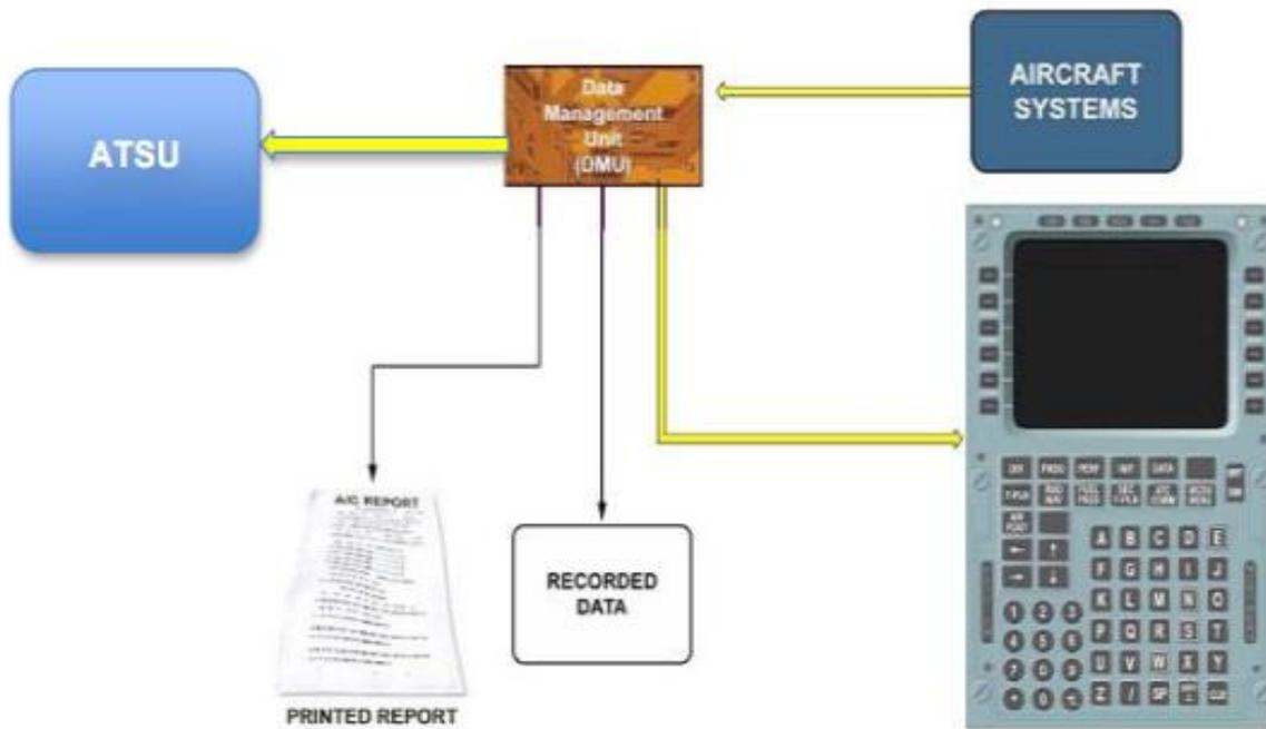
Figure 5: Function of the DMU
